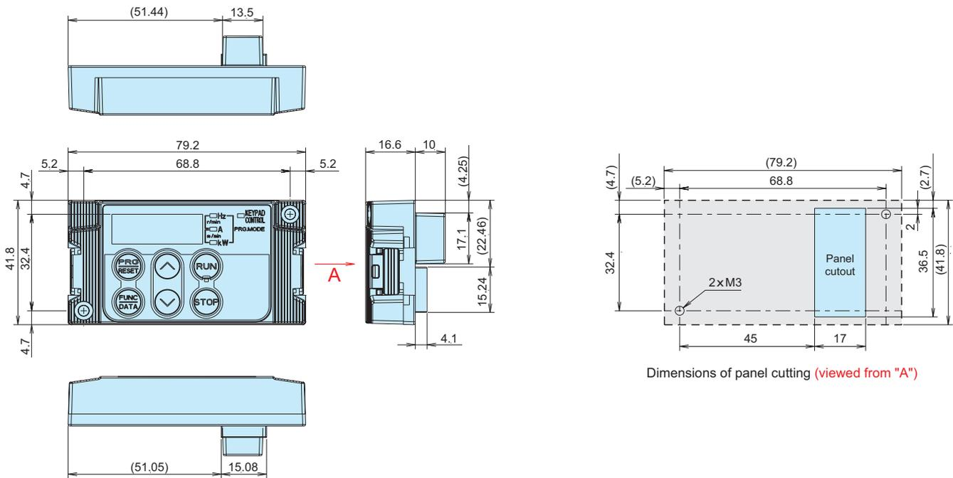
\* Dimensions when installing the supplied rear cover
