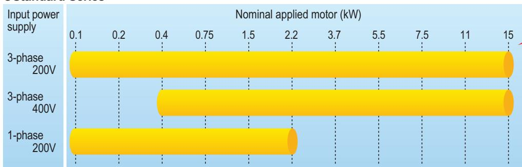
Capacity expanded to 15kW
