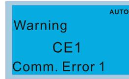
1. Press the STOP / RESET key to reset the fault code. If there is no response, contact your local distributor or return the unit to the factory. To view the fault DC bus voltage, output current and output voltage, press MENU and then choose 6: Fault Record.
