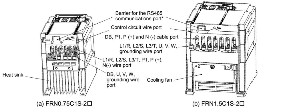
(\*When connecting the RS485 communications cable, remove the control circuit terminal block cover and snip off the barrier provided in it using nippers.)
