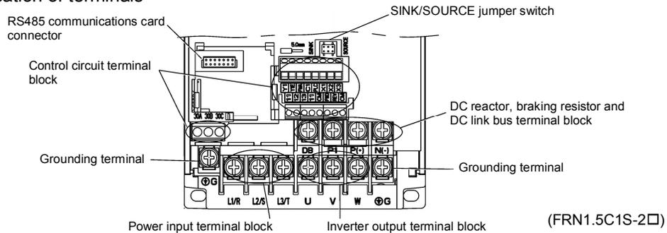
Figure 2.3 Enlarged View of the Terminal Blocks
