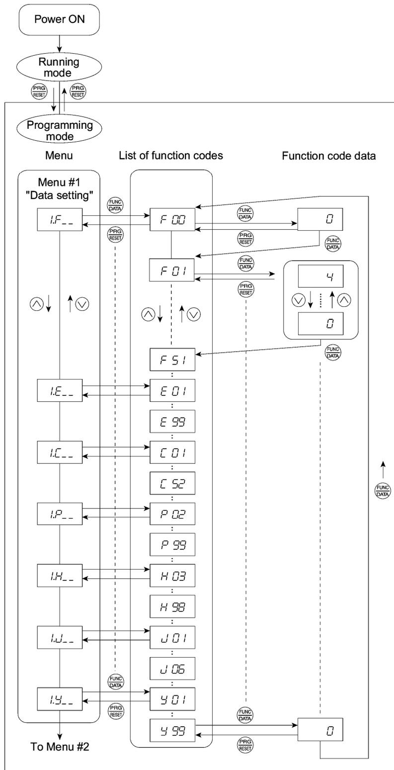
Figure 3.4 Status Transition Diagram for "Data Setting"
