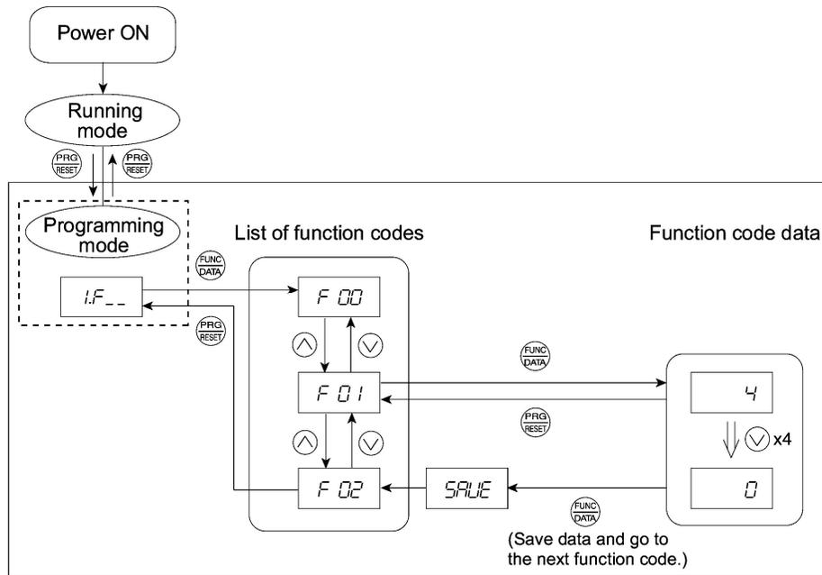
Figure 3.5 Example of Function Code Data Changing Procedure
